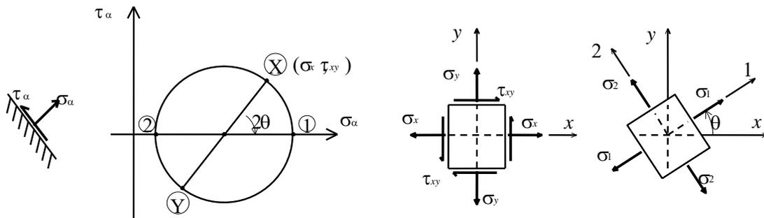
Tensiones principales:  $\sigma_{1,2} = \frac{\sigma_x + \sigma_y}{2} \pm \sqrt{\left(\frac{\sigma_x - \sigma_y}{2}\right)^2 + \tau_{xy}^2}$
